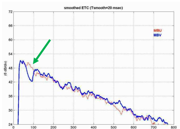
Figure 5. Scale model impulse responses with stage reflector (red) and without (blue), measured from B1 (cellos) to M2 (trumpets)
